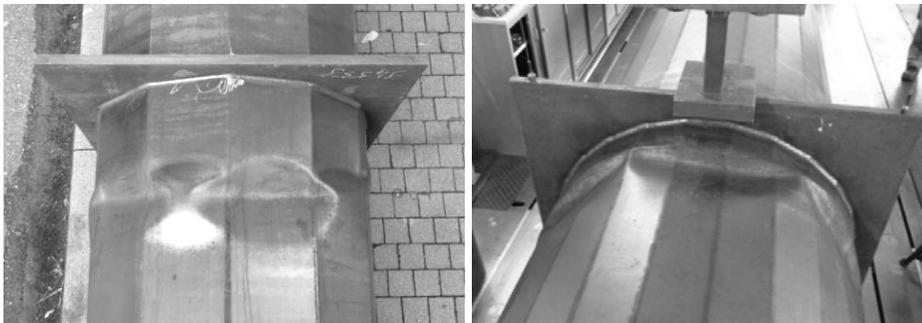
*Fig. 2:* left: polygonal section with 12 corners, local buckles between two adjacent corners; right: polygonal section with 24 corners, buckles throughout several corners
